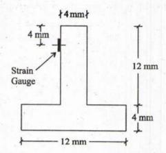
A small T-section is used in inverted position as a beam and is shown in figure over a span of 400 mm. If due to the application of forces shown, the longitudinal strain gauge at F registers a compressive strain of 1500 microstrains, determine the magnitude of P. Take E = 200 GPa.
