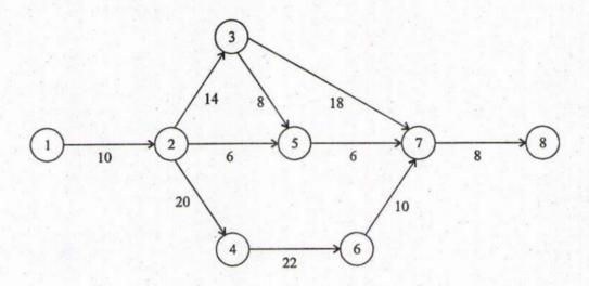
Identify the critical path in the network as shown in figure and determine the project completion time. The duration are in weeks.
