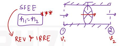
In a steam turbine with steam flow rate of 1 kg/s, inlet velocity of steam of 100 m/s, exit velocity of steam of 150 m/s, enthalpy at inlet of 2900 kJ/kg, enthalpy at outlet of 1600 kJ/kg, the power available from the turbine will be nearly
