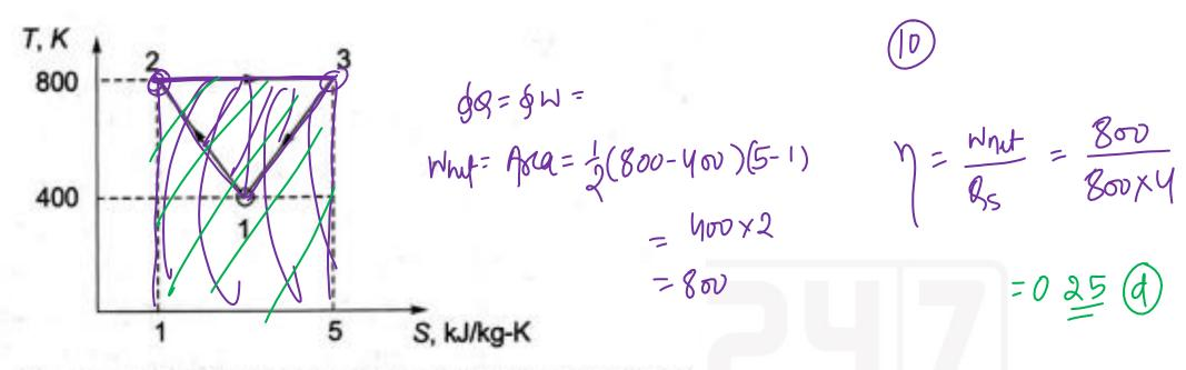
The thermal efficiency of the hypothetical heat engine cycle shown in the given figure is
