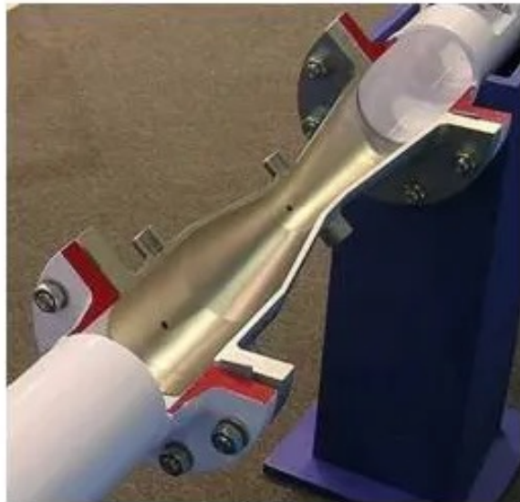
Cut-View of a Venturimeter
