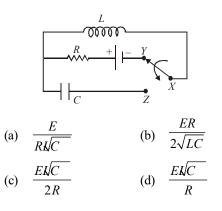
3. In the circuit shown, the symbols have their usual meanings. The cell has emf *E*. *X* is initially joined to *Y* for a long time. Then, *X* is joined to *Z*. The maximum charge on *C* at any later time will be
