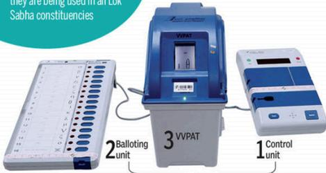
1 & 2 are joined by a cable. Taken together, the system is called EVM
