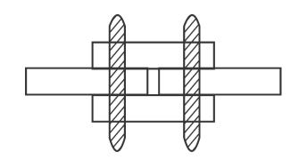
$\rightarrow$  in double cover butt joint connection is not eccentric
