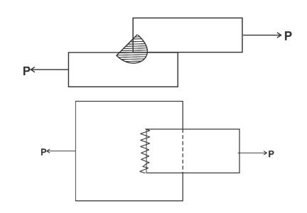
$\rightarrow$  fillet weld failed due to shear failure
