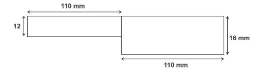
Strength of butt weld =  $L \times t_{min} \times \sigma_{SP}$ = 110×12×142 = 187.44 kN
