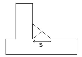
$\rightarrow$  Size (S) in the fillet weld is indicated by side of the triangle of fillet
