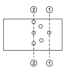
Width of plate = b Diameter of rivet = d Strength of plate at (1) - (1)
